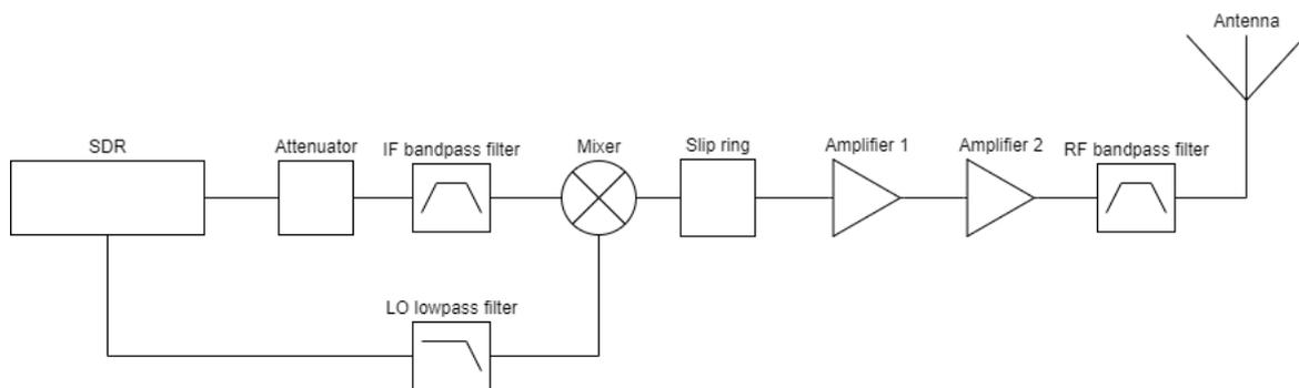
Figure 5.4: Simple transmitter design.
