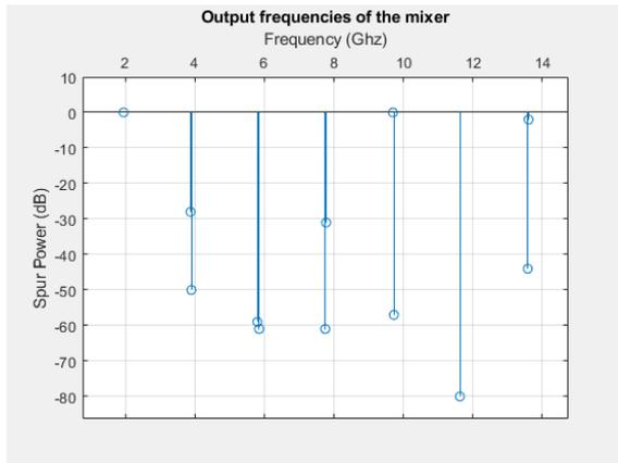
Figure 6.2: Output of the mixer with a desired frequency of 9.7 GHz.
