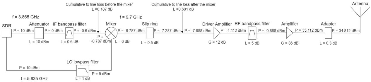
Figure 7.2: Link budget of the improved Slotted Waveguide antenna transmitter chain.
