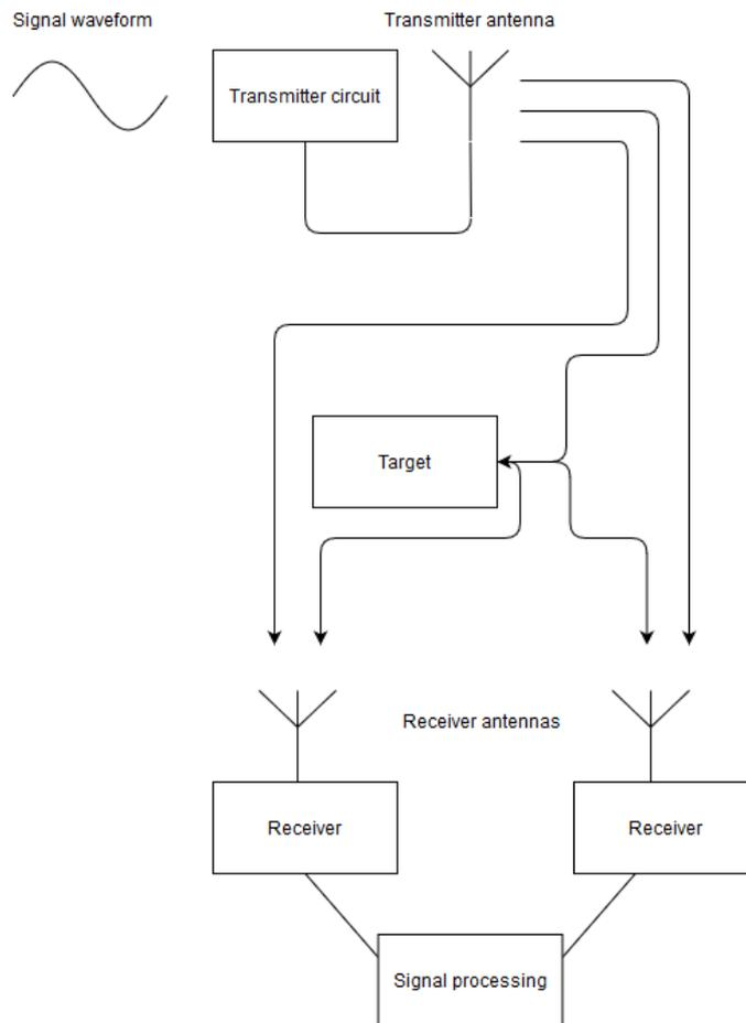
Figure 1.2: Diagram of the bi-static radar
