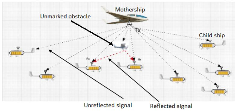
Figure 1.1: Visualisation of the bi-static radar in combination with drones.
