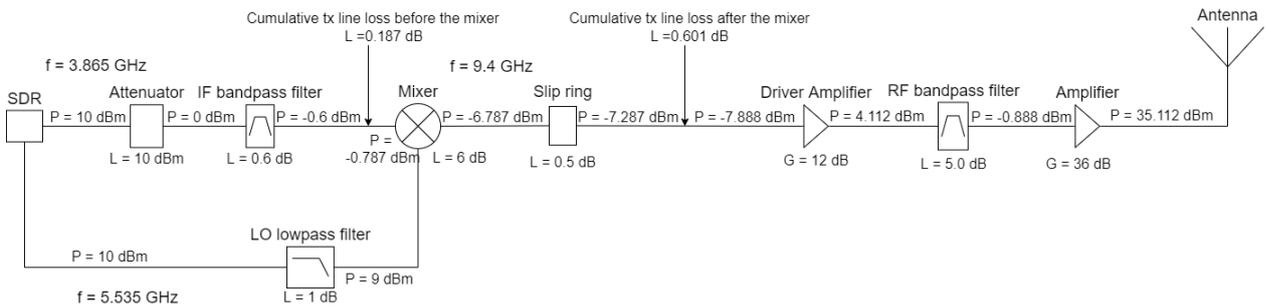
Figure 7.3: Link budget of the MetaSensing antenna transmitter chain.
