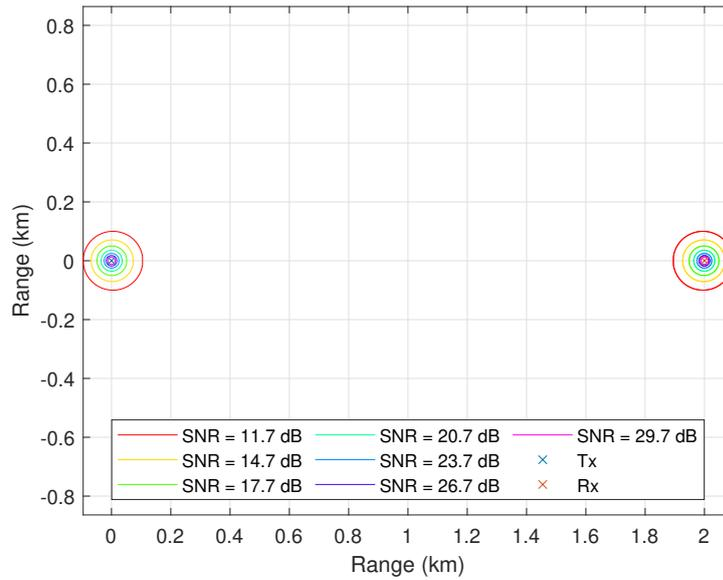
Figure 7.6: Cassini ovals range  $L = 1 \text{ km}$  (baseline range) and  $R_{tx} = 100 \text{ m}$  (target to receiver range)
