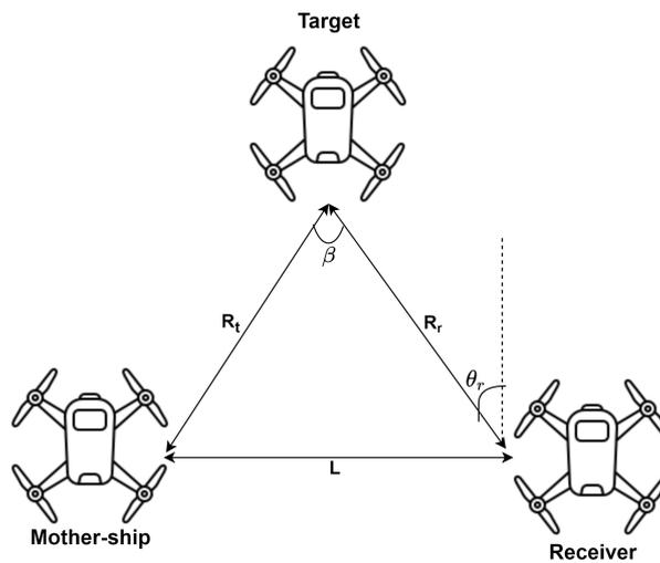
Figure 4.1: Bi-static radar configuration.
