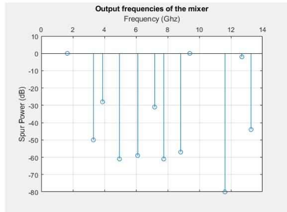
Figure 6.3: Output of the mixer with a desired frequency of 9.4 GHz.
