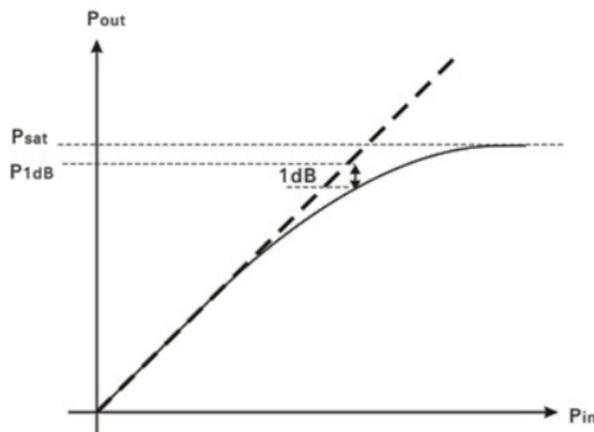
Figure 5.3: Power saturation of weakly nonlinear device.
