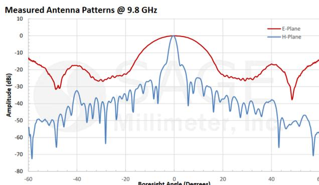
Figure 6.4: The radiation pattern of the Slotted Waveguide Antenna
