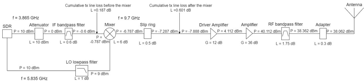
Figure 7.1: Link budget of the Slotted Waveguide antenna transmitter chain.
