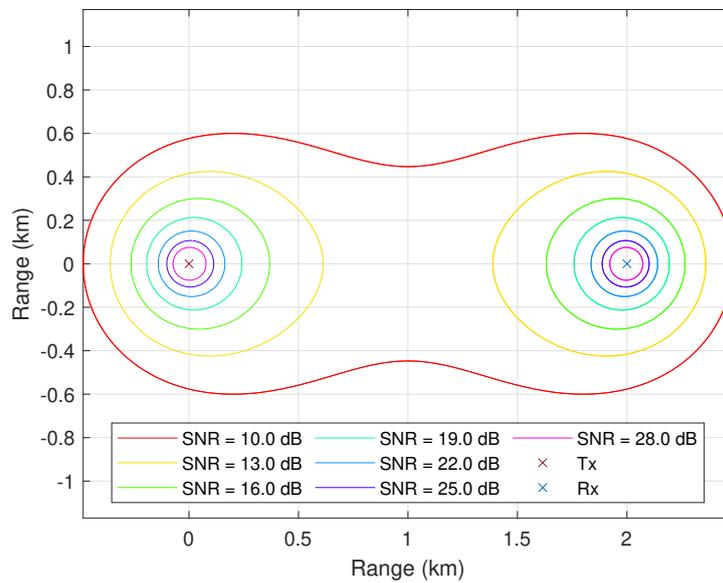
Figure 7.7: Cassini ovals range  $L = 2 \text{ km}$  (baseline range) and  $R_{tx} = 600 \text{ m}$  (target to receiver range)
