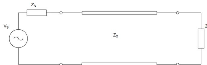
Figure 5.2: Simple transmission line.
