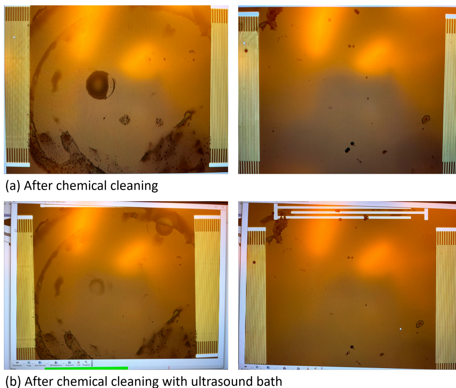
Figure 11.3: PM loading devices (a) after chemical cleaning, (b) after chemical cleaning with ultrasound bath
