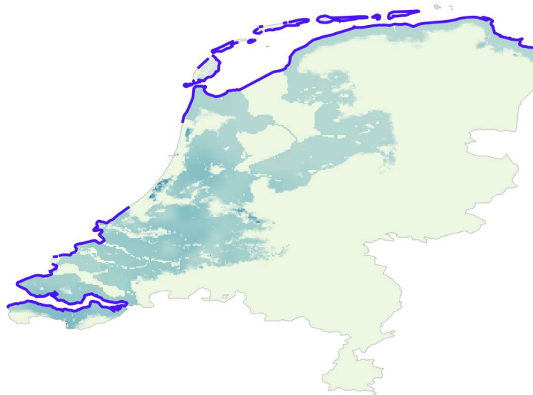
Figure 4.4: The coast reinforcement map of the Netherlands for RCP8.5 with RP1000 years in 2080 for the 50 th percentile.
