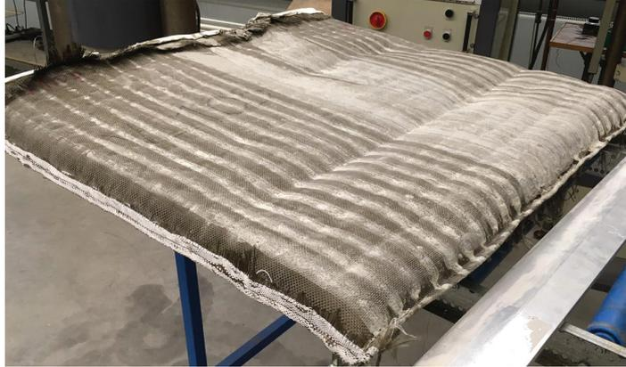
FIG. 13 First demonstrator made of single-curved basalt spacer fabric
