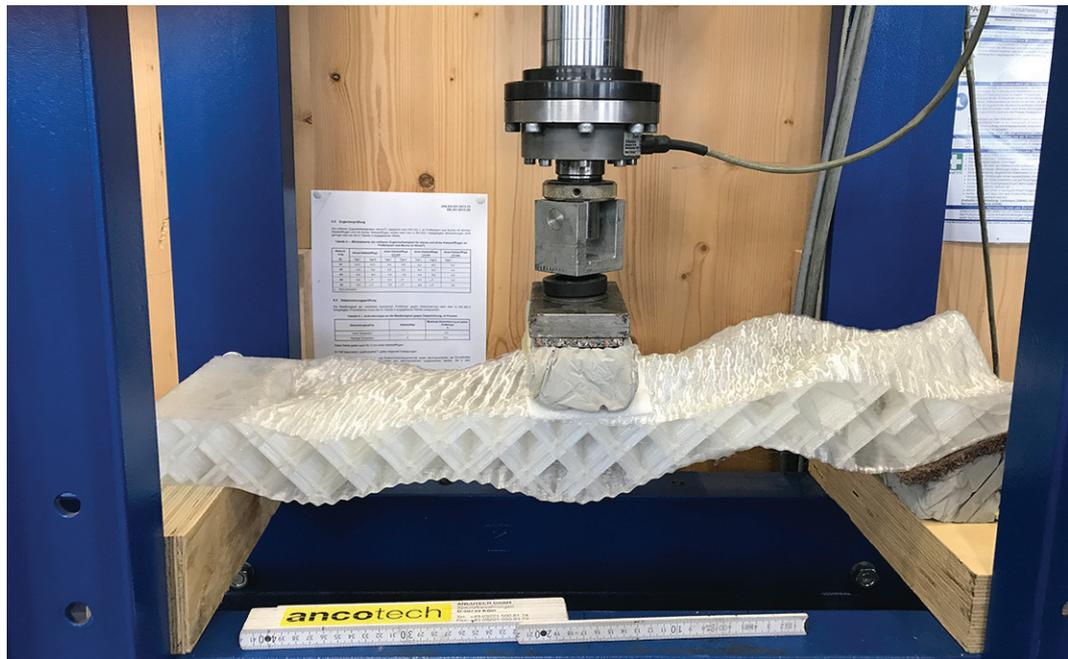
FIG. 5 Design of the experimental unit with test specimen, distributor plate and support forms
