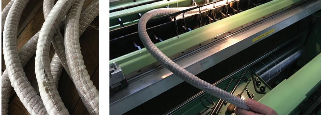
FIG. 8 PCM Strands close-up with Kemafil® casing (left); Yarn processing on coarse warp knitting machine (right) © Christiane Sauer
