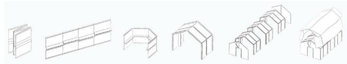
FIG. 20 zelthaus.com, research results from the PET area are used for self-supporting, insulated temporary buildings
