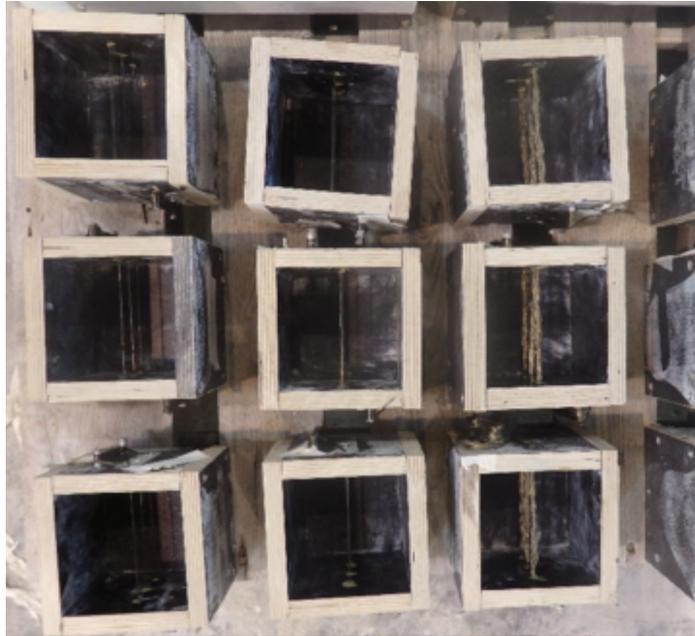
FIG. 7 Single rovings in form-work for pull-out tests
