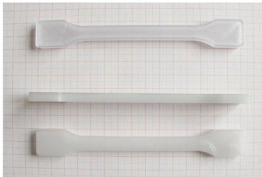
FIG. 3 3D printed test specimen tensile test
