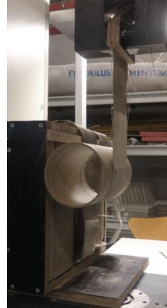
FIG. 8 Single-layer basalt fabric, test setup – peel-off test
