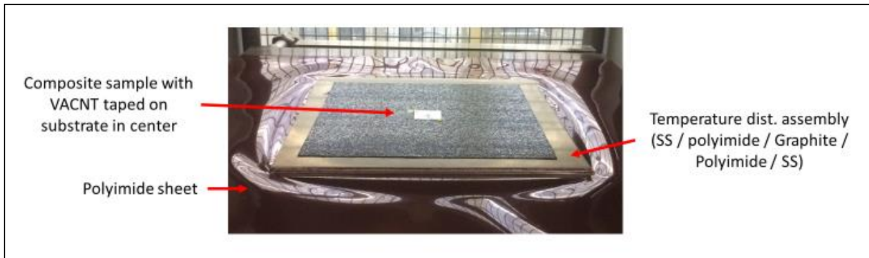
Figure 17 - Composite specimen placed on lower temperature distribution assembly
