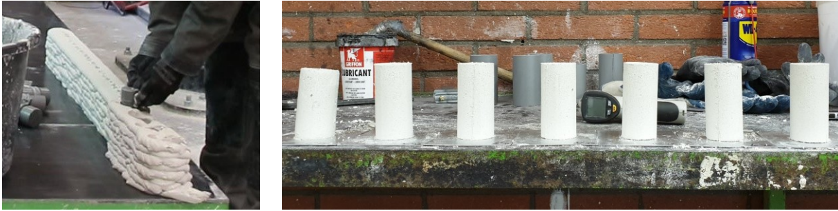
Figure 26: Left: extracting samples by pushing a mould into the print. Right: demoulded samples ordered in age from left to right (0, 15, 30, 60, 90, 120 and 180 minutes) during testing of the proof of concept.
