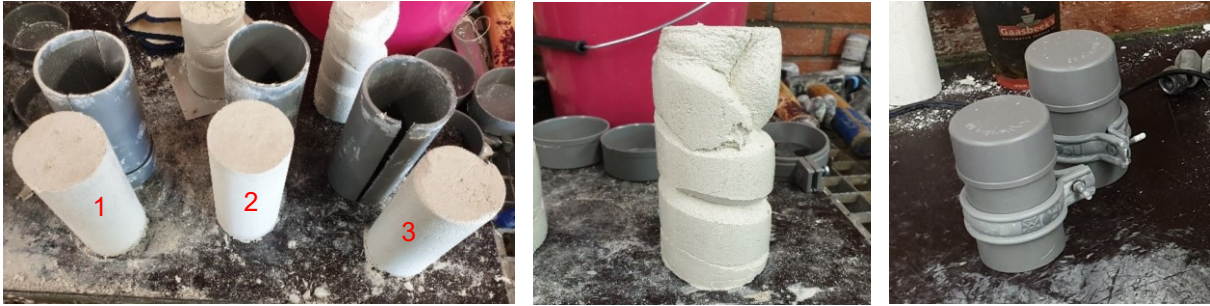
Figure 25: Left: three different mould configurations. Middle: distorted sample. Right: final mould configuration.
