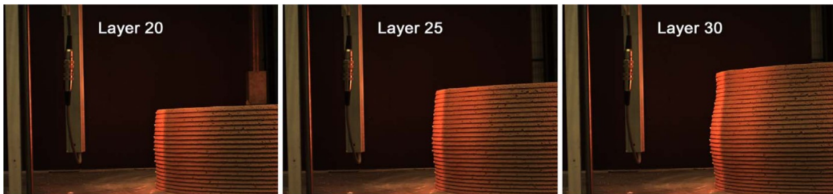
Figure 14: Deformed shape of a cylinder during printing. Reproduced from [11].
