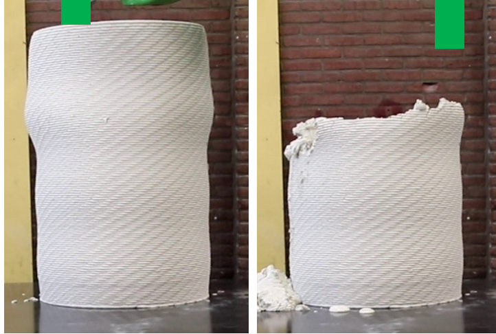
Figure 53: Print C2 before collapse and after collapse printed at 15.08 s. per layer on day H4.
