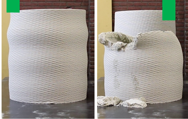
Figure 52: The moment before collapse and the collapsed cylinder C1 printed at 18.74 s. per layer on day R2.
