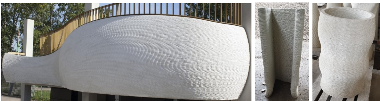
Figure 15: Several prints produced by Bruil. Left: full size mock-up-up of a balustrade of a balcony for the renovation of an apartment building in Den Helder. Middle: unsuccessful print of a U-shaped wall which has locally buckled at the bottom. Right: a curvy cylindrical column, demonstrating the capabilities of printing structures with strong curvatures in the vertical plane.
