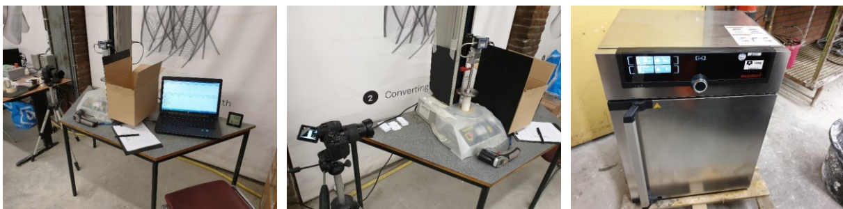
Figure 24: Left and middle: setup of the uniaxial compression test. Right: the oven in which the samples are stored.
