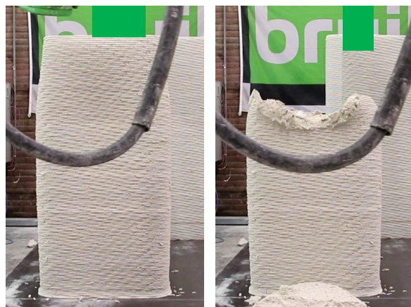
Figure 56: Typical deformation behaviour before failure of print S1. Picture shows the print printed at a speed of 8.40 s. per layer.
