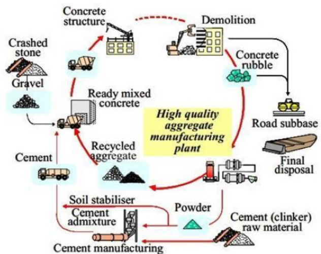
Figure 2.21 Process of concrete recycling. Retrieved from (Ganiron, 2019).
