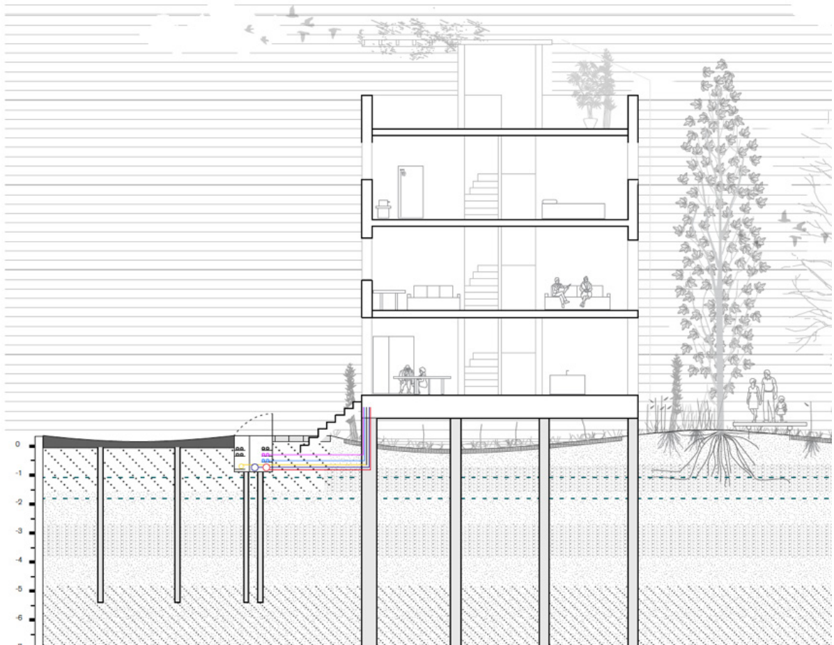
Fig 4.16 The public space is natural and will subside. The buildings are on piles and designed with the flexible entrance to the subsiding public space. Infrastructure and subsurface infrastructure are also founded on piles to prevent breakage and high maintenance costs by subsidence (drawing by Filippo Laflaur).
