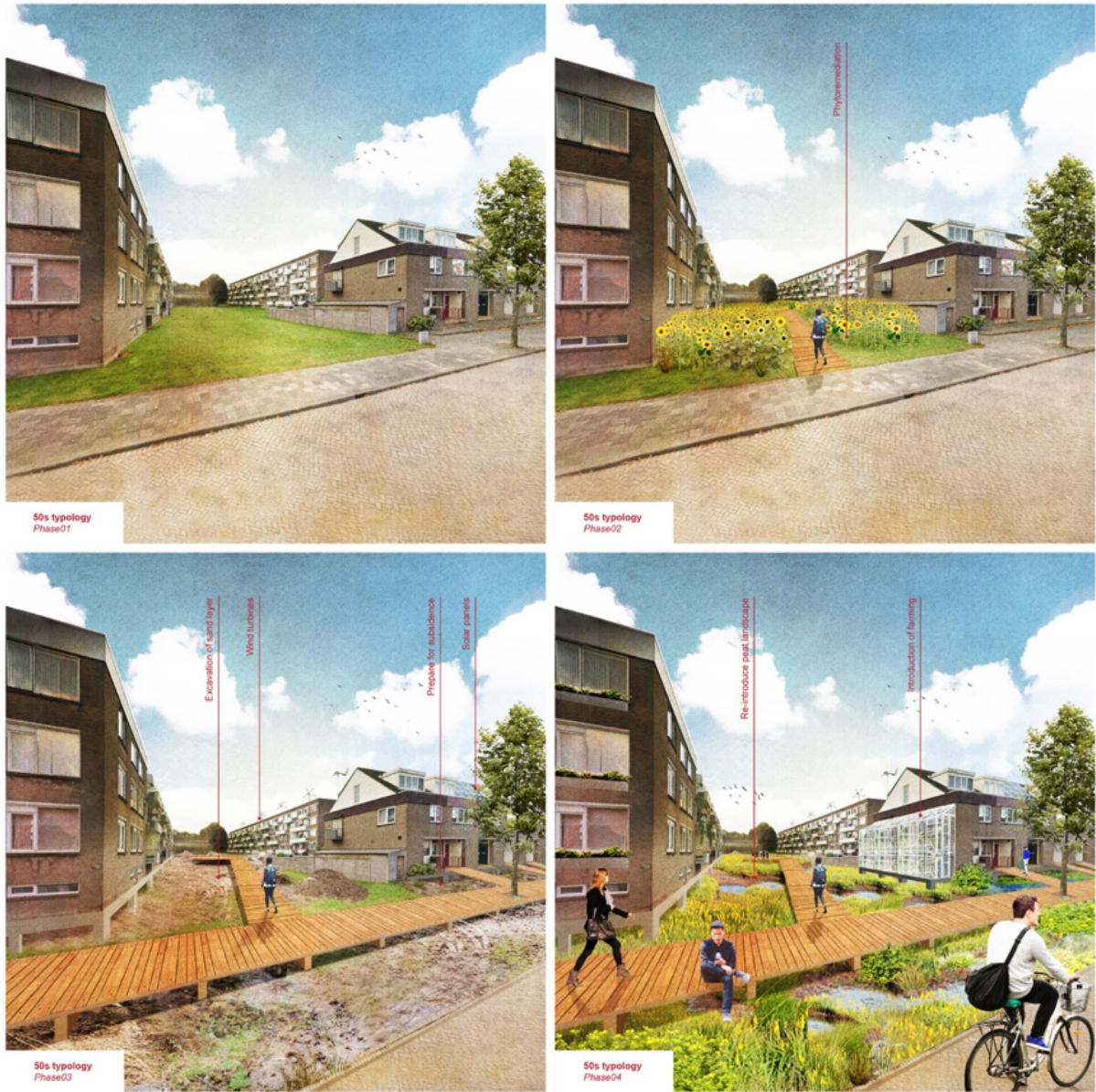
Fig 4.22 Phase one is the original state. In phase two the first step is implementing GRO to clean soils and to stop adding sand to mitigate effects of subsidence. This is done differently in phase 3 by stimulating the restoration of the endogenous ecosystem and design the buildings on piles so that they can function with subsiding soils.
