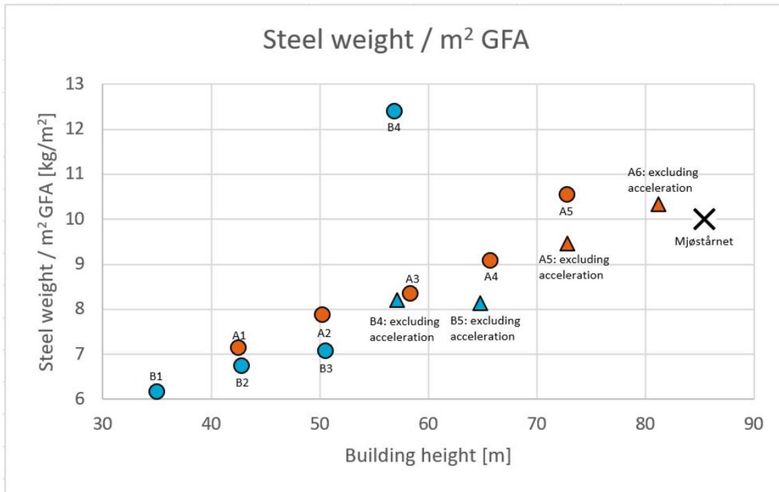
Figure 6.33: Steel weight per m² GFA compared to reference project
