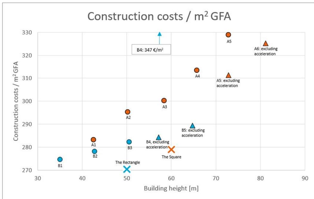
Figure 6.35: Construction costs per  $m^2$  GFA for building types A and B
