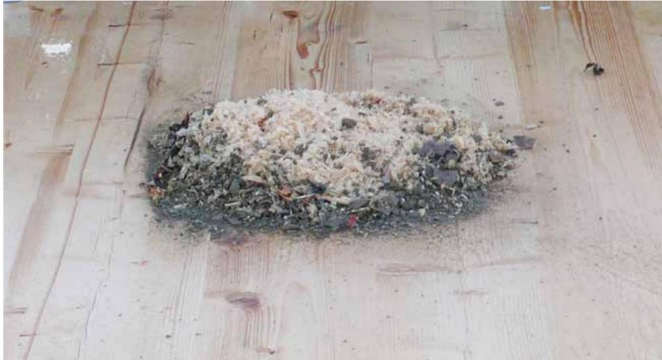
Figure A.6: The total collected waste after a week of erection of the CLT frame at Murray Grove [14].
