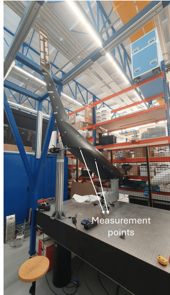
Fig. 5 GVT measurement points
