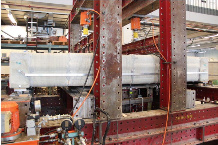
Fig. 2.6 Scale model in 4-point bending test set-up
