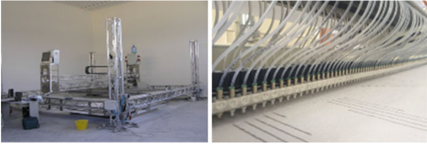
Fig. 2.14 D Shape ® 3D-printer (left) and print head (right) (Lowke et al. 2018)
