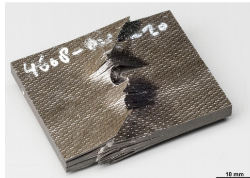
Figure 4.2: OHC specimen after testing
