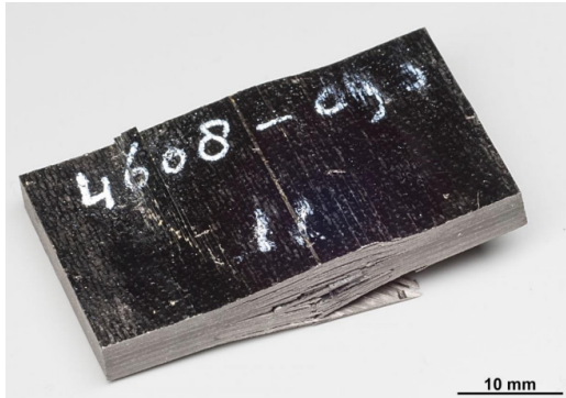
Figure 3.4: Example of 90° compression specimen after testing.
