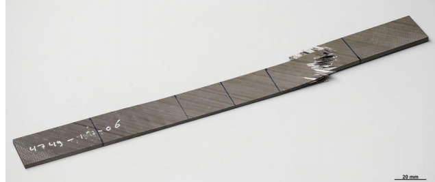
Figure 3.5: In-Plane Shear (IPS) specimen after testing.
