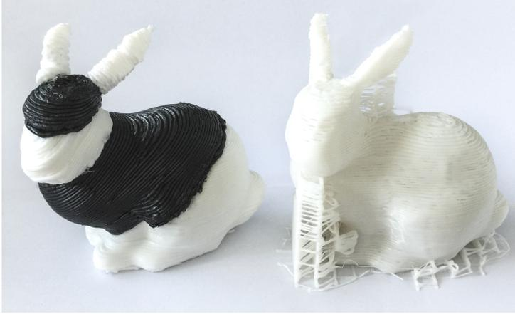
**Figure 2.1:** A bunny model fabricated by our RoboFDM (left) vs. the model made by conventional FDM (right). Note that, to illustrate our decomposition algorithm, different parts of the bunny model being fabricated along different directions are fabricated by filaments in different colors.
