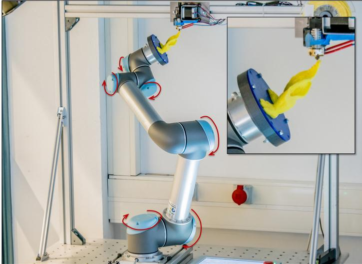
**Figure 3.12:** The hardware of our robot-assisted AM system using a 6-DOF robotic arm, where each red arrow indicates a motor to provide one rotational DOF. The extrusion head is fixed in our system so that the orientation change for material accumulation is realized by moving the end effect of the robot arm inversely.
