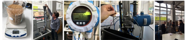
Fig. 6-10. Weighing and dosing pellets. Differential pressure. Releasing trapped air from the sensor. PBL class instructions at QMUL.
