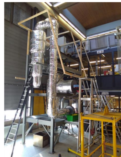
Figure 3.9 (a) Separation of fines and lights from moist crushed concrete on-site (W. de Vries, PhD-thesis TU Delft) & (b) HAS - Heat treatment of fines and lights (industrial prototype at 3 tons/h at the TU Delft lab).
