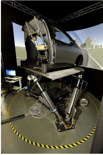
Fig. 3. Delft advanced vehicle simulator.
