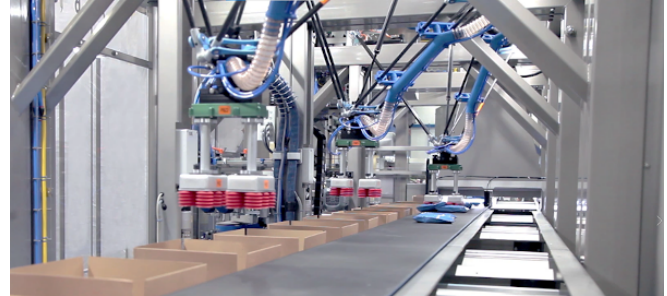
Fig. 1: An industrial secondary packaging solution where robots coordinate to pick and place products into packaging boxes.
