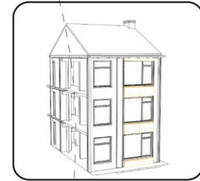
PLACING THE JAMB EXTENSIONS AND THE UNDER THE WINDOWS PANELS
