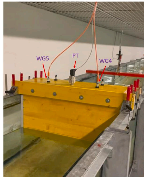
(b) Box OWC placed in tank - WG4 and WG5 are wave gauge designated by orange wires and PT is the pressure gauge depicted by the black wire
