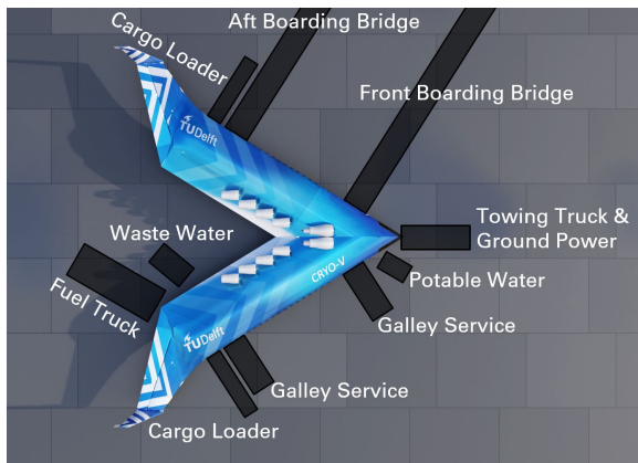
Figure 11.1: Gate position layout of the Cryo-V
