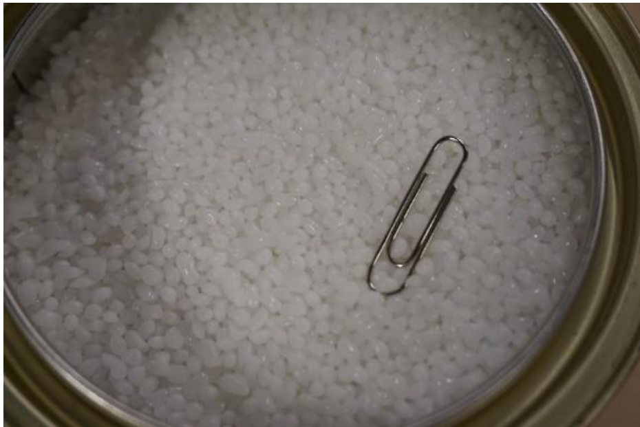
Figure 3. 5: The wax-based warm mix additive used in this study.
