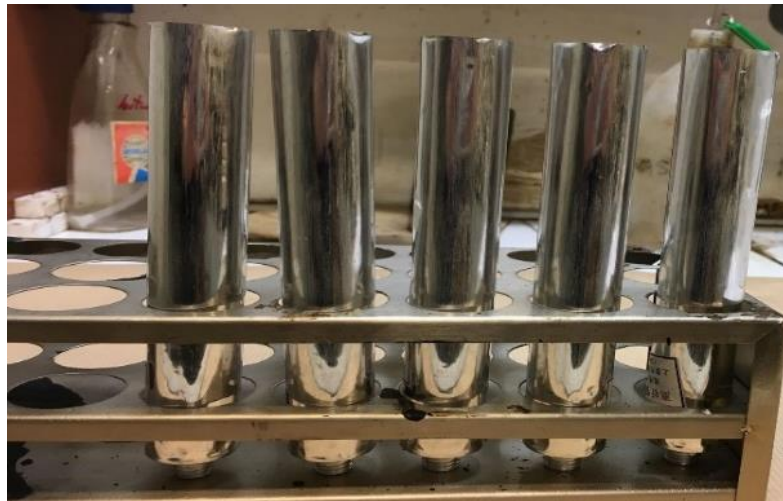
Figure 8. 1: Arrangement of separation tubes in vertical orientation.
