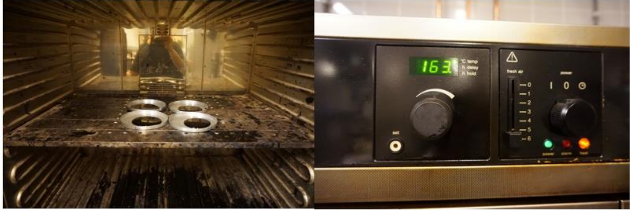
Figure 3. 11: The modified static oven aging simulation
