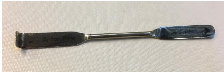
Figure 7. 7: Anton Paar spatula for sample trimming.
