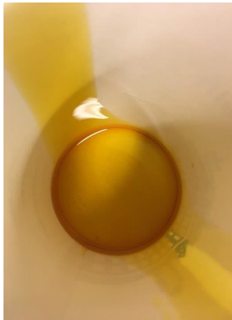
Figure 3. 6: The chemical-based warm mix additive used in this study.
