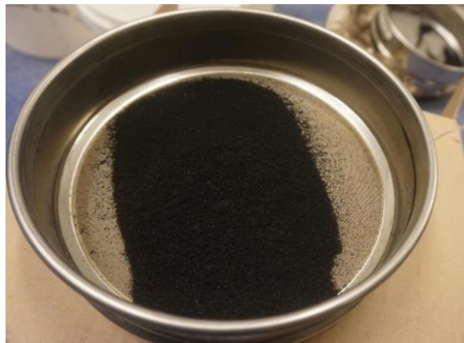
Figure 3. 2: Crumb rubber modifier with particle sizes ranging from 0 - 0.5 mm.
