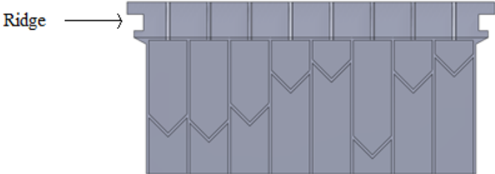
Figure 16: Cross-sectional view of the lattice structure of one wall of the metamaterial showing random cavity depths. In addition, the ridge for sliding the metamaterial wall into the frame is marked
