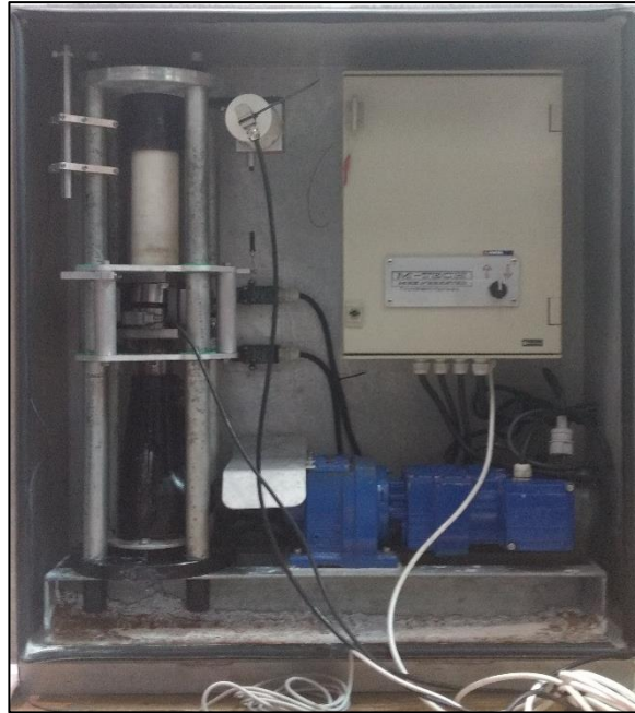
Figure 3.8 KOMPIS , with clockwise from the specimen: draw wire sensor, control box, electrical engine, load cell and newly installed strain sensor.
