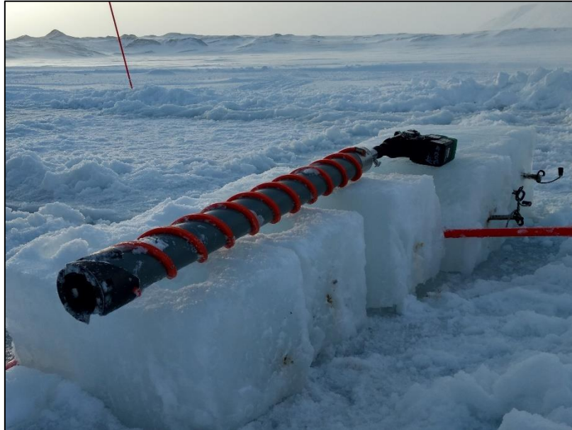
Figure 3.4 Coring system and retrieved blocks of sea ice (Svea, Svalbard) from which horizontal cores were drilled
