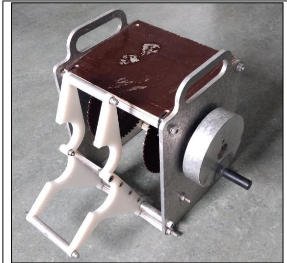
Figure 3.6 Saw box used for cutting specimens with parallel faces and normal to the longitudinal axis
