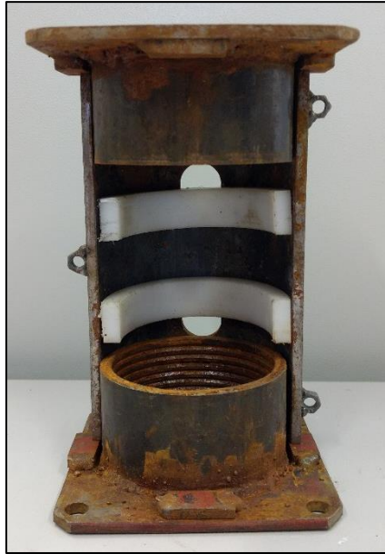
Figure 3.7 Two end caps and one mantle showing the inside of the system. During operation two mantles were applied
