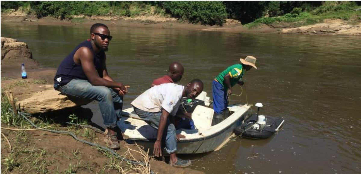
Figure 7: Preparation of an ADCP measurement at Mushumbi Bridge
