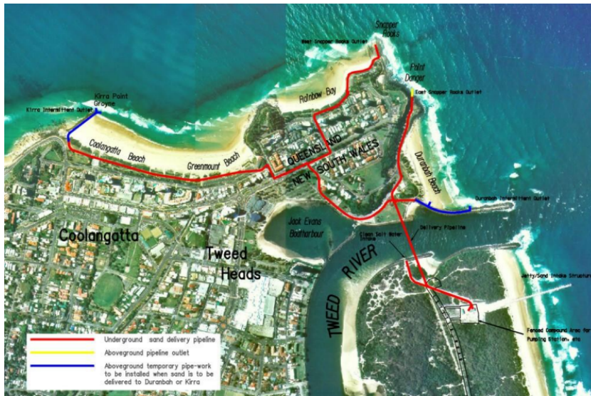
Figure 3.3: Tweed river sediment bypass system overview Soares, 2017
