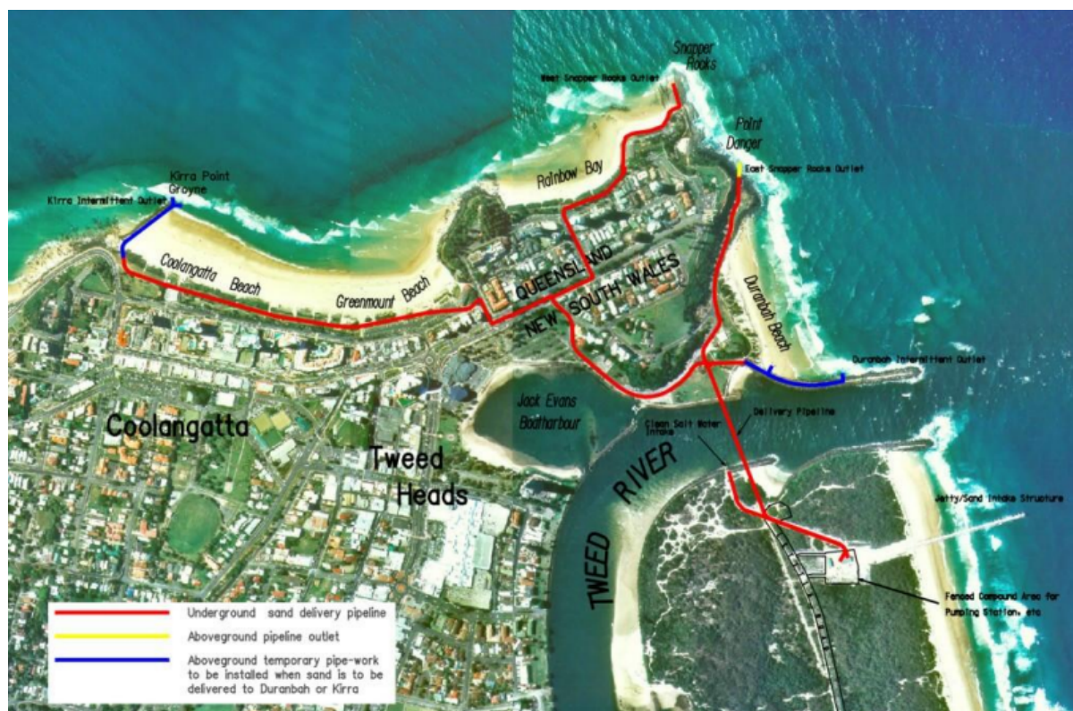
Figure C.3: Tweed river sediment bypass system overview Soares, 2017
