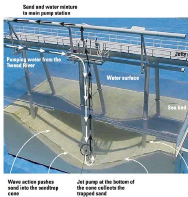
Figure C.4: Tweed River Entrance Sand Bypass Project, sediment collecting system overview (Ware, 2016)
