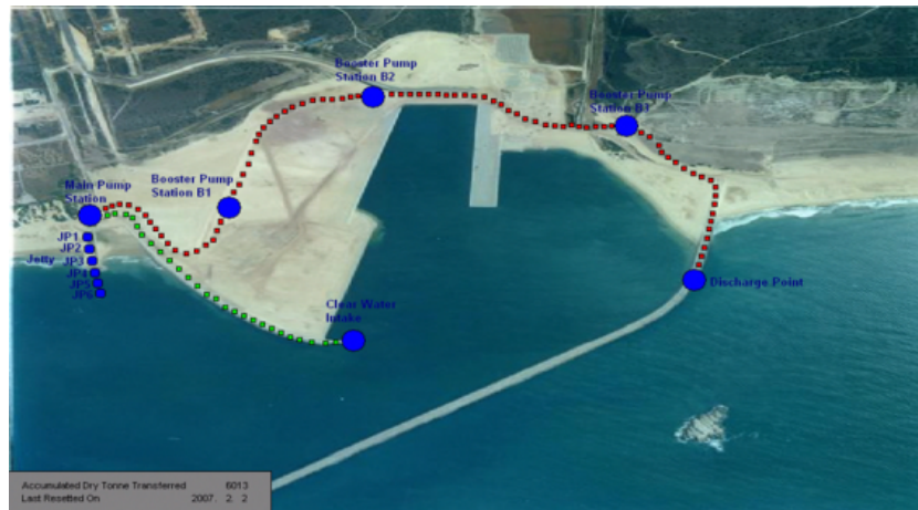
Figure 3.5: Schematic view of Port of Ngqura Sand Bypass system (Soares, 2017)
