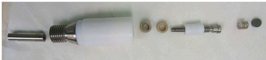
GRAPHICAL ABSTRACT | By modifying a rotating disc electrode, permanent magnets could be positioned very close to the electrode surface.
