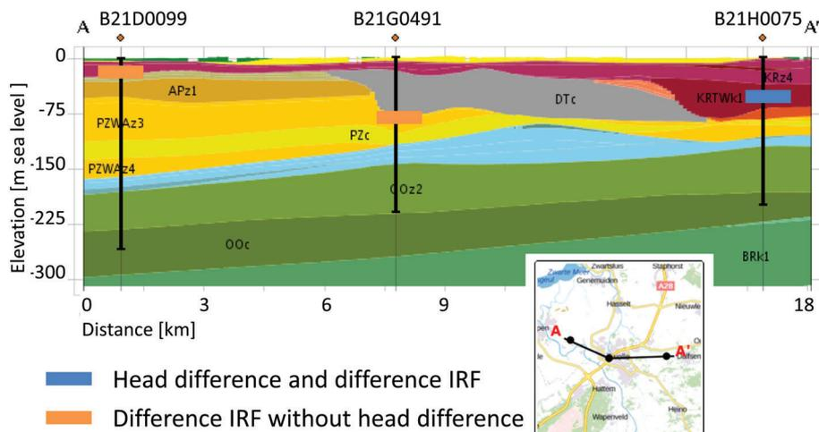
**Figure 4.** Cross section around Zwolle showing locations of observation wells and the hydrogeological model REGIS II with geological formations (capitals) and aquifer (z), aquitard (k), and complex (c) hydrogeological units.
