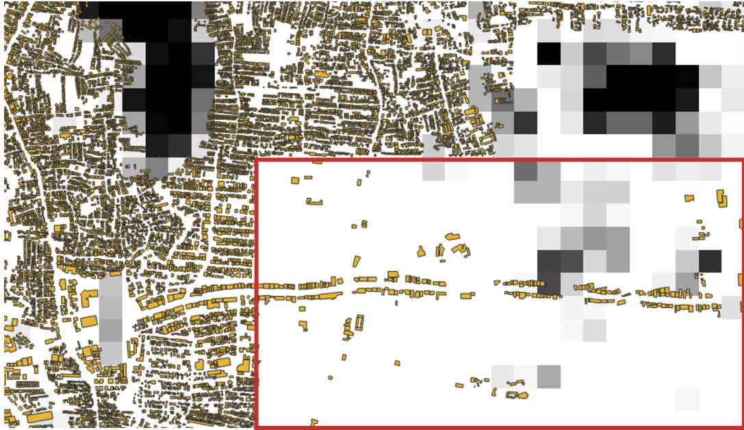
Figure 4: The OSM building footprint map (highlighted yellow) overlaid with the Copernicus built-up area map (grayscale). The grayscale blocks represent the built-up area data grid squares of 100m x 100m. The red box indicates an area that should be built up according to the Copernicus built-up area map, but with many mapped OSM building footprints absent. This indicates incomplete OSM data in that area.
