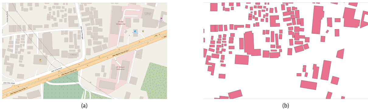
Figure 1: Complete OSM map of an area in Denpasar, Bali (a), and the isolated building footprint polygons (b).
