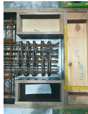
(c) Detail of reinforcement in element RAQTAN_1-A .
