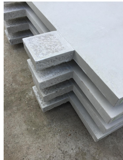
Figure 6.4: The cast landing platforms. (source: Rempt van der Donk)
