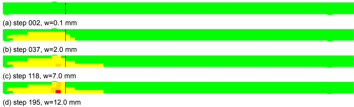
Figure 9.20: Strain states for marked steps. Blue is a strain below 0.0001, green below 0.1, yellow below 0.3, orange below 2.0 and black otherwise.
