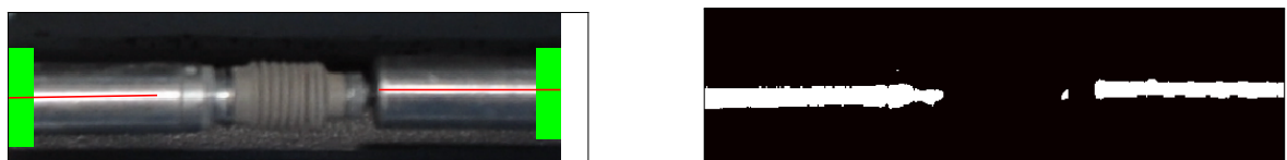
Figure 10.22: The analysis on the photos to determine the elongation. The shimmer on the metallic cylinders is traced by setting a threshold on the whiteness (right image). The direction can be determined by finding the first and the last white pixel for each cylinder (resulting in the red lines in the left image). The intersection point is located where the left red line intersects the normal to the right red line. The used Python code is attached in Appendix D.2.
