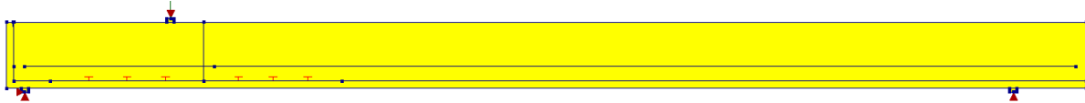
(b) The model for the RAQTAN_2-B and RAQTAN_3-B elements, without stirrups and with modifications.
