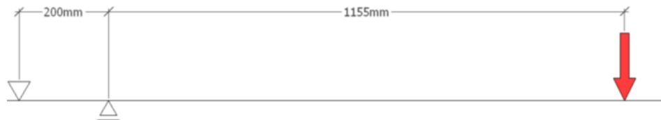
Figure 6.6: Used model of the Raqtan landing platform to the wall. The red arrow indicates the influence of the dowel connection.
