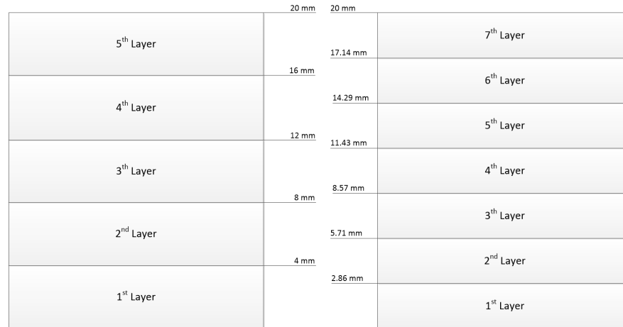
FIGURE 3.2: Multi-layered sample preparation sketch of A. dense samples, and B. loose samples.
