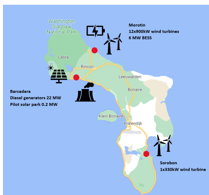
Figure 1.2: Map of Bonaire with the solar pilot and the diesel generators located on the west side of Bonaire at Barcadera. On the north side of Bonaire at Morotin 12 wind turbines are located (900 kW each), together with the battery energy storage system (BESS). Lastly, in the south of Bonaire, one single wind turbine is located at Sorobon.
