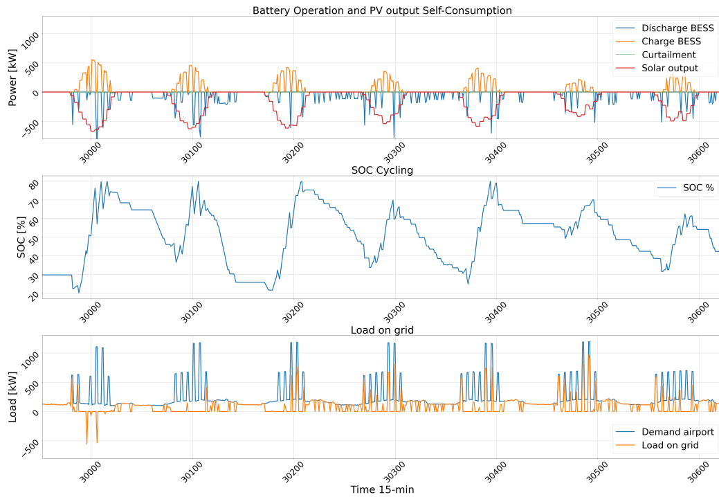
Figure 4.7: The battery charging profile of a 2000kWh/1000kW BESS in combination with a 1000 kWp solar park controlled by Self-Consumption. The upper graph represents the (dis)charging behavior of the battery and the PV electricity production (negative). The graph in the middle provides the resulting SOC-cycling of the BESS. Lastly, the total demand profile of the airport and the net grid load are given in the graph at the bottom.
