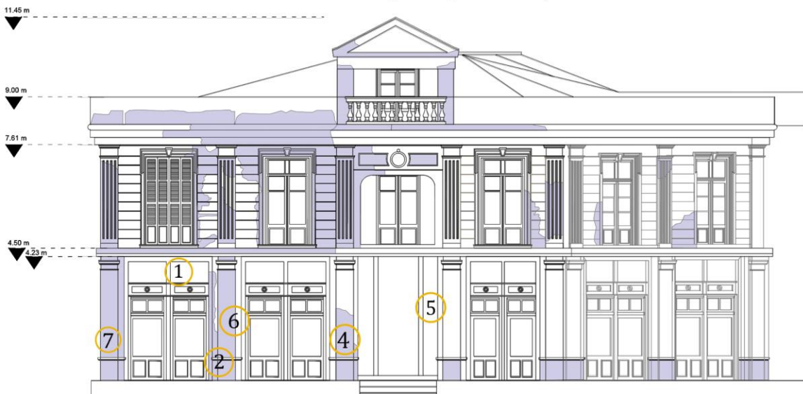
Damage registration (Survey Product)
