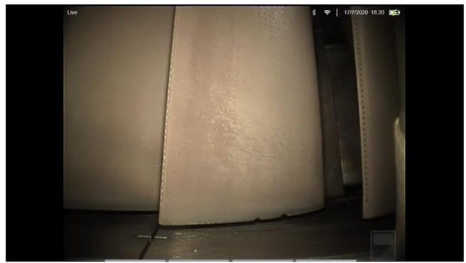
(b) A frame taken out of another example borescope inspection video. It shows a textureless surface of the blades.
