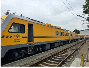
Fig. 12 XLN4C-01 inspection vehicle.
