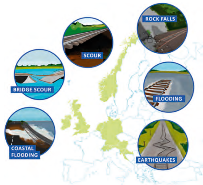
Fig. 1. Different types of failure on railway infrastructure [10]
