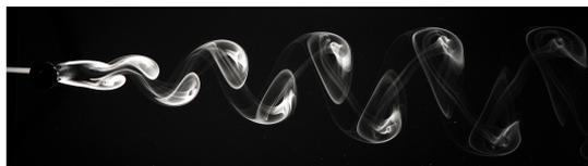
Figure 2.1: Visualization of the vortex street behind a circular cylinder in air [1]
