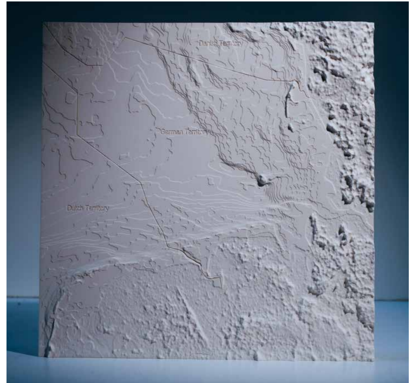
The Altitudes of Flatness, Thinking with Sections and Models Course, Year 2020-21. Horizontal scale (x) 1:750.000. Vertical scale (y) 1:7500. Model size 500 x 500 mm.
