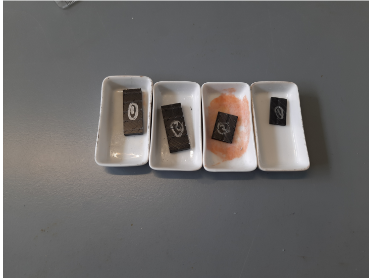
Figure 5.9: Composite Specimens Ready to be Put in Furnace
