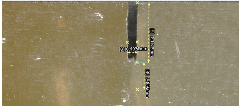
Figure 4.8: SENB Specimen with Crack Dimensions Observed Through Microscope
