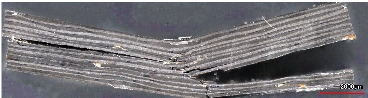
Figure 6.9: A Stitched Cross-Section of VDE-Composite Specimen After ILSS Test
