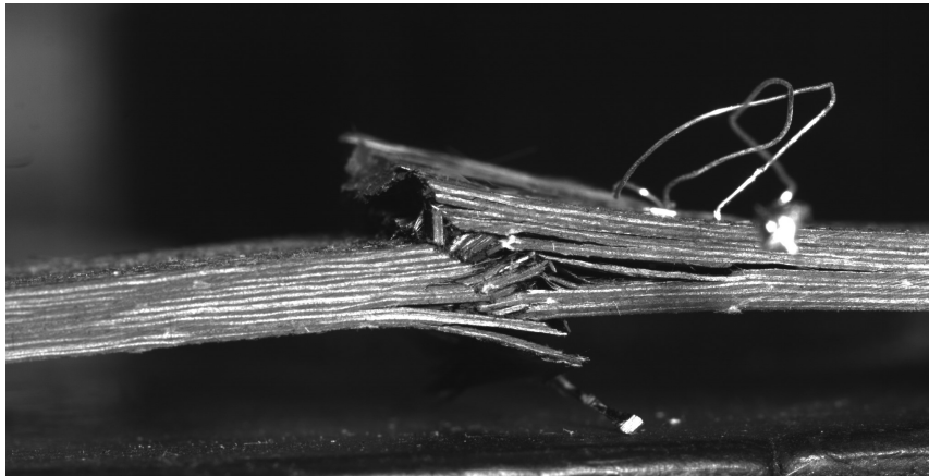
Figure 7.6: Compression Failure for a BADGE-DDS Sample
