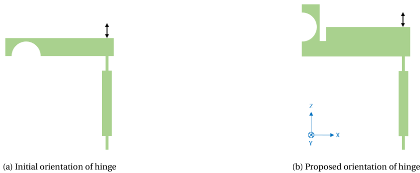
Figure 4.25: Schematic of flexural elements
