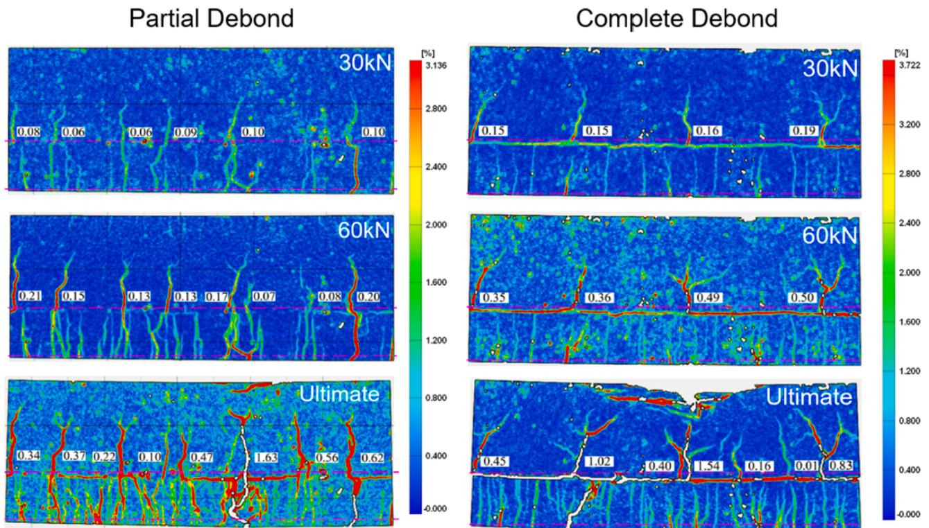
**Fig. 10.** Development of cracks in the constant moment region of Partial Debond and Complete Debond at 30kN, 60 kN and ultimate load. The dashed horizontal lines show the section where crack widths are measured in SHCC and in concrete.
