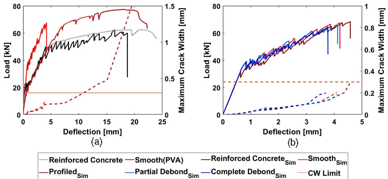
Fig. 17. (a) Numerical and experimental response of Reinforced Concrete and Smooth(PVA). (b) Numerical response of all the hybrid beams.
