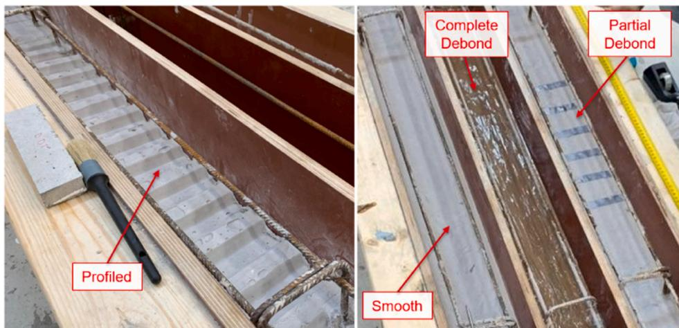
Fig. 3. Interface preparation of the hybrid beams before casting the concrete top layer.
