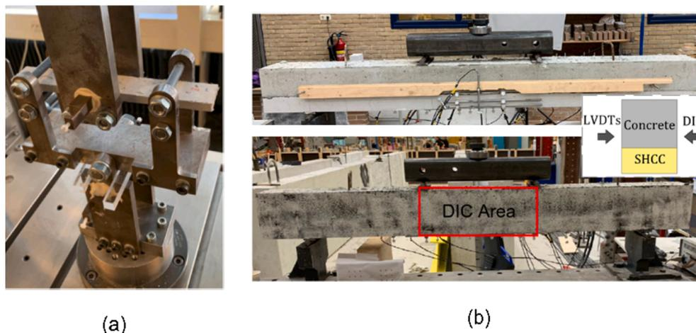
**Fig. 4.** Test setup for (a) material tests for the effect of fibre types in SHCC and (b) structural tests with LVDT measurement on one side and DIC on the other. DIC results discussed in this paper correspond to the constant moment region of the beam, as demarcated in red.
