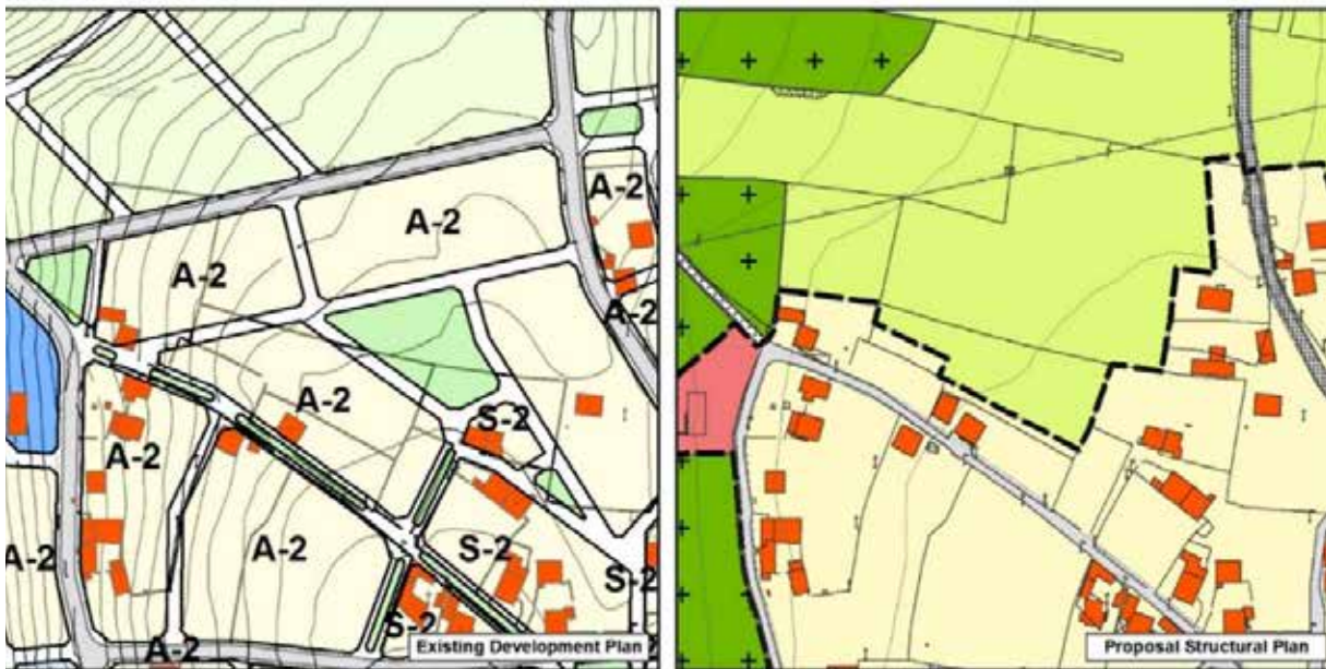
FIGURE 6 Settlement morphology was developed as enabling sustained agricultural production. An approach for conserving cadastral roads and ownership patterns was adopted in the structural plan, unlike the development plan.
