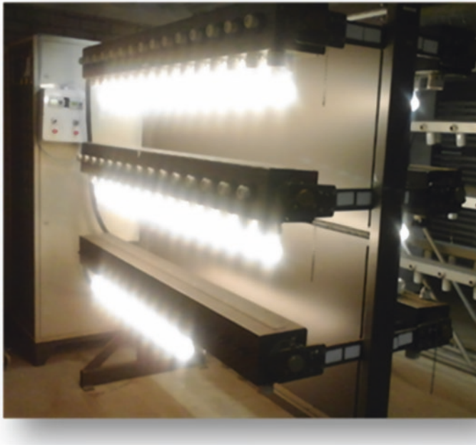
Fig. 7.12 Lifetime tests with glass LED bulbs put into traditional burning racks
