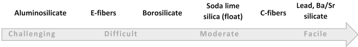
Fig. 22 Recycling by kiln-casting ease based on the chemical composition of the tested glasses
