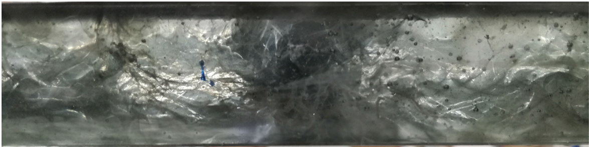
Fig. 20 Kiln-cast beam from manually sorted CRT screens, prepared at 870 °C (10 h)
