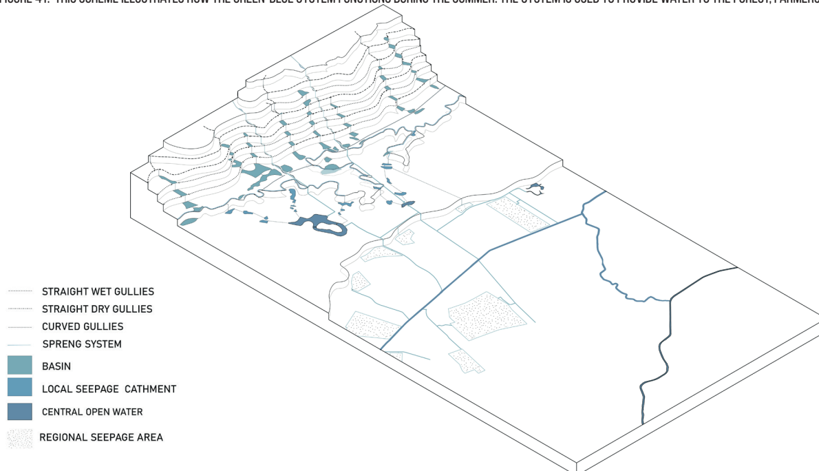
FIGURE 41: THIS SCHEME ILLUSTRATES HOW THE GREEN-BLUE SYSTEM FUNCTIONS DURING THE SUMMER. THE SYSTEM IS USED TO PROVIDE WATER TO THE FOREST, FARMERS AND LOCALS.
