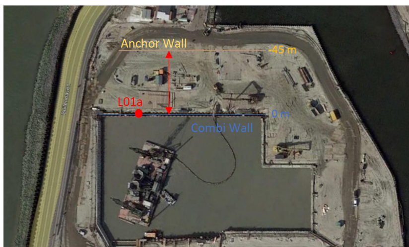
Figure 2.6.1: Top view of the outer lock head with reference dimensions. [Google Maps]
