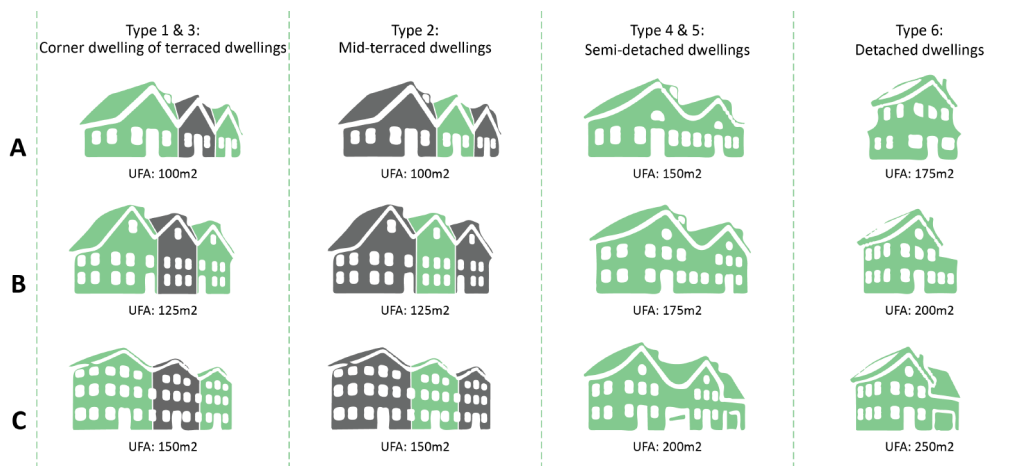
Figure 57: Three sub-types for each archetype gives 12 dwelling types in total. Sub-types differ in the amount of UFA (own illustration).
