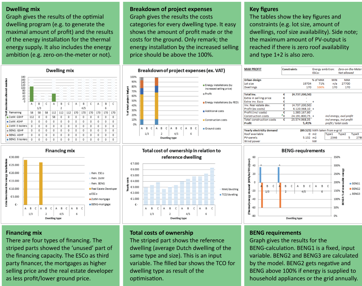
Figure 59: Dashboard as output result of the model. The example used shows the results for the case study of 'Het Verborgen Geheim' to realize a zero-on-the-meter energy ambition (see 'energy ambition' within the constraints in the top right). In this case the possibilities to increase the selling price or involve an ESCO were disabled (see 'financing mix'). It also looks like if there is a negative energy demand, however, this means that energy is supplied to the grid annually. This counts for the time of installation. The amount gets lower during the years due to degradation of the PV-panels. (own illustration).
