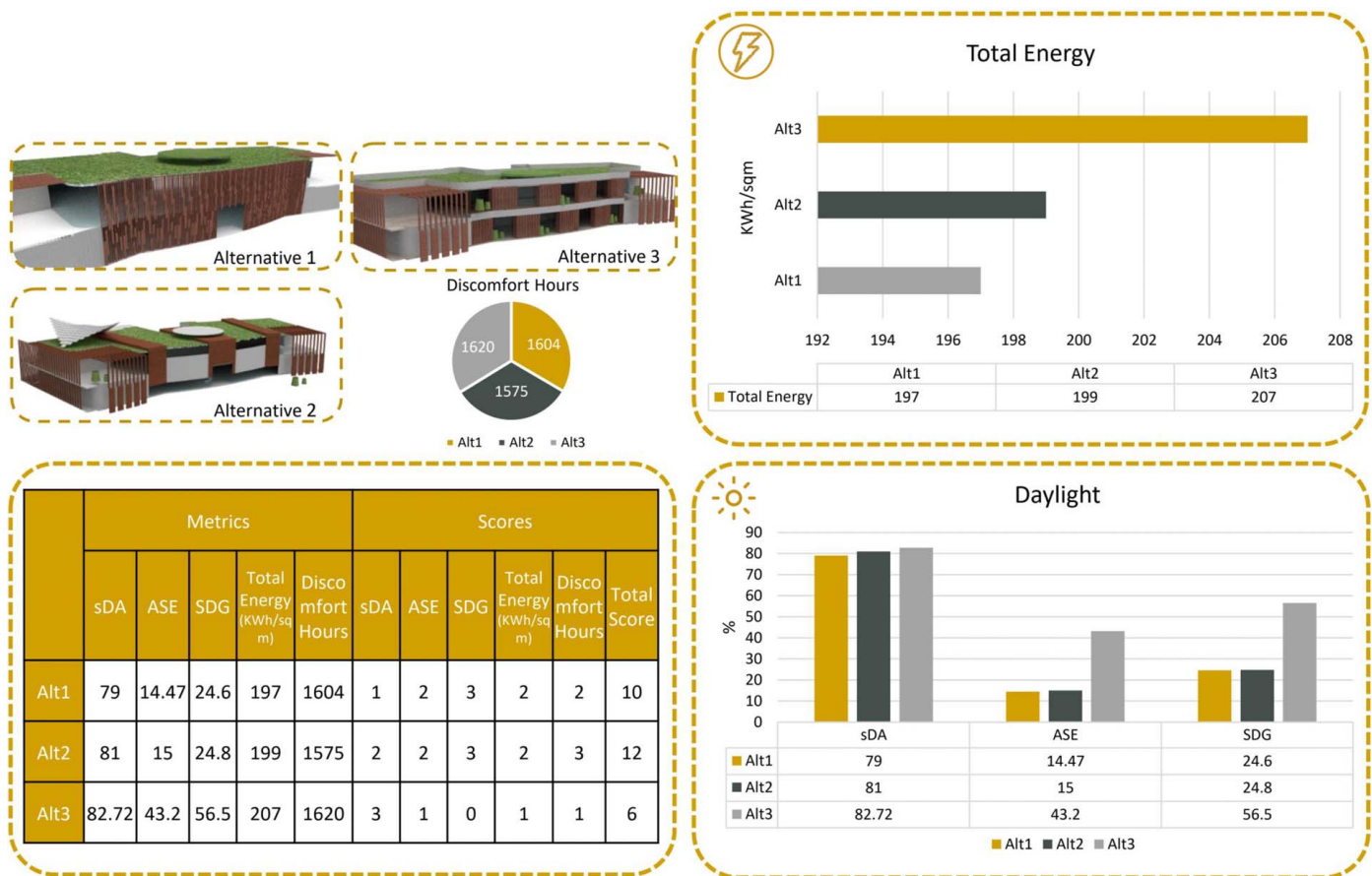
Fig. 7. Facade design – Performance analysis and evaluation of the commercial building; Urmia team.
