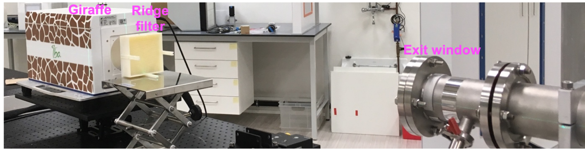
Figure 3.14: Picture of experimental setup for SOBP measurements. Ridge filter can be seen in front of the Giraffe detector.
