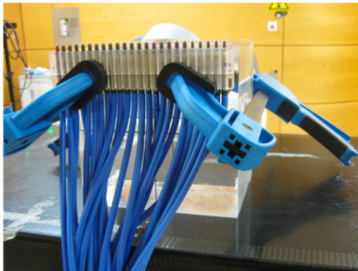
Figure 2.4: Setup of measuring lateral beam profiles in air with 24 PinPoint ICs by Schwaab et al. [38].
