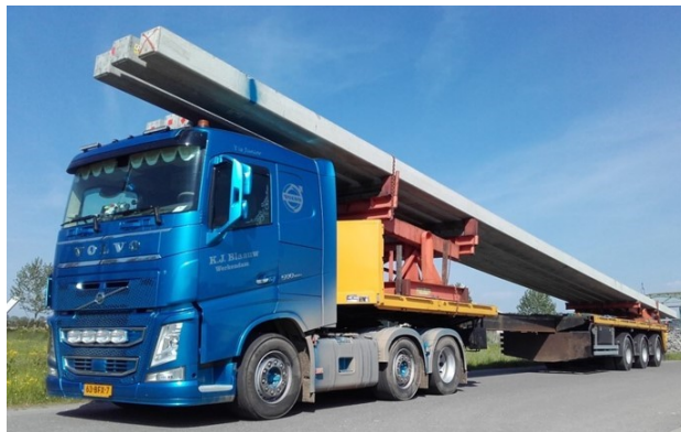
Figure 2.13: Large transport prefab pile of 27.5m [18]
