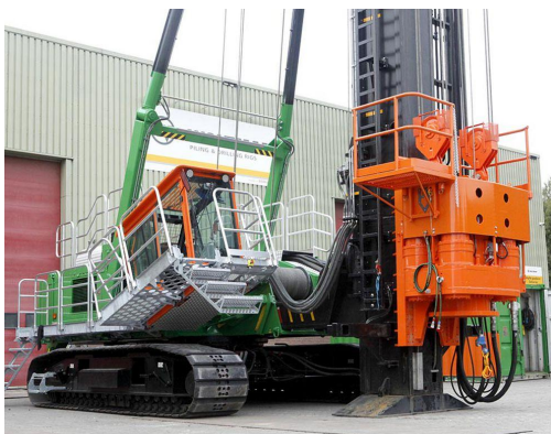
Figure 2.14: Larger electric piling rig of BAM, Woltman 90DRe [7]
