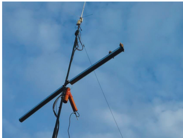
FIGURE 4: The adapted shorted dipole and the ITA LWA II 20-meter-long wire antenna (from top to lower right).
