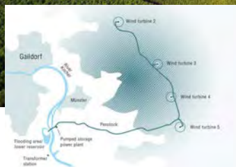
Wind turbines connected to a hydro-electric power plant by a channel to the valley [Max Boegl Wind]
